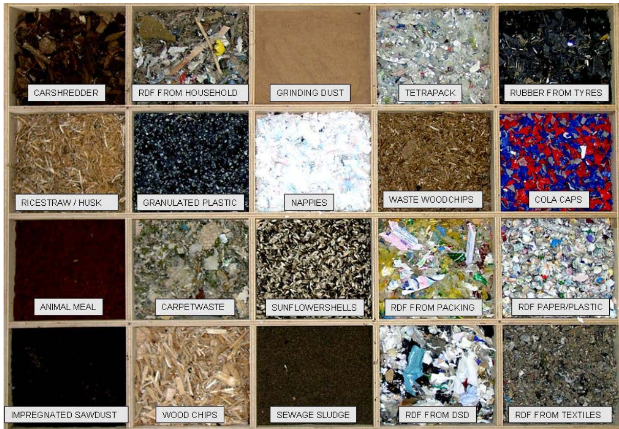
Figure 5-2 Assortment of alternative fuels used in the cement industry (source: FLSmidth Pfister GmbH)
