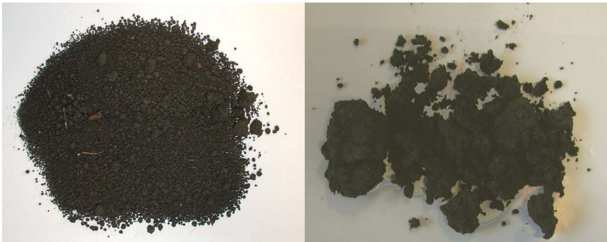
Figure 5-5 Left picture: dried sewage sludge pellets (dry matter content > 85%); Right picture: Mechanically dewatered sewage sludge (dry matter content < 30%)
